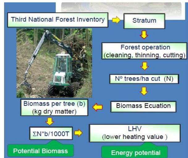
Fig. 4. Schematic diagram of the methodology
