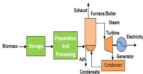
Fig. 1. Direct Combustion/Steam Turbine System
