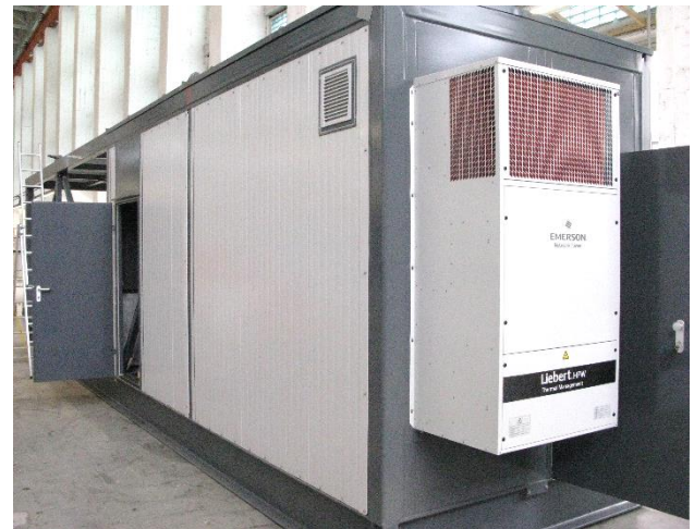
Fig. 5. Right side of the measurement container with indoor part where the ester filled tank will be installed
