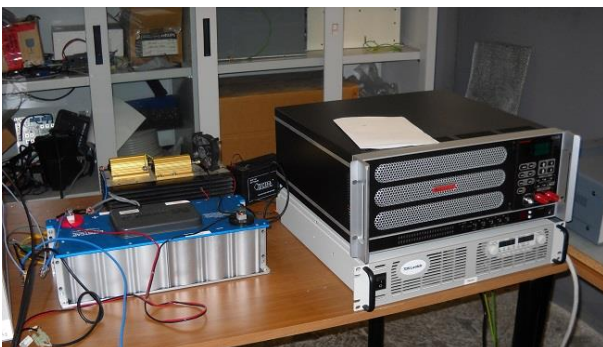
Fig. 5: maxwell supercapacitor (left) with the electronic load and the power supply (right)
