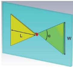
Fig.6: Bowtie nanoantenna coupled with MOM diode [21]
