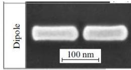
Fig.2: Dipole nanoantenna [5]
