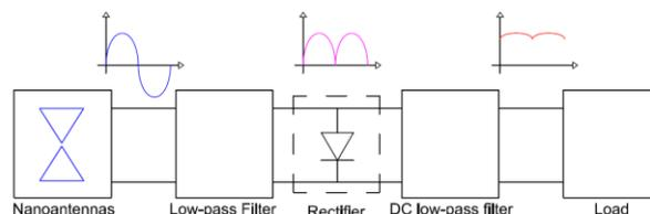
Fig.1: Block diagram of infrared nano-rectenna
