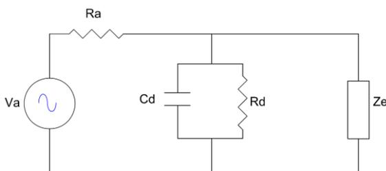
Fig.10: Equivalent circuit of a solar rectenna
