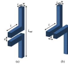
Fig.4: Dipole nanoantenna terminated by travelling wave MIM plasmonic waveguides: (a) vertical coupled strips, (b) lateral coupled strips [19]
