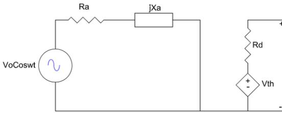
Fig.9: Electric equivalent circuit of the antenna-coupled thermocouples
