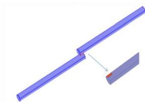
Fig.3: Dipole nanoantenna coupled MIM diode [17]
