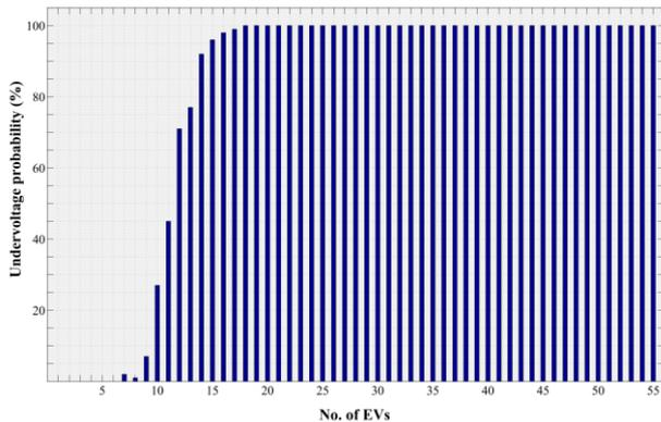
Fig. 4. Voltage violations (%) vs. No. of EVs.
