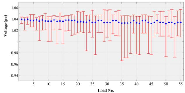
Fig. 3. Voltage range at service points w/o EV.
