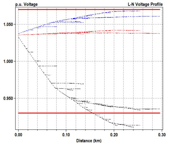
Fig. 5. Voltage profile at 9 pm with 18 EVs.
