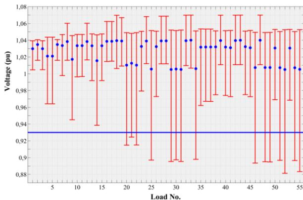
Fig. 6. Voltage range at service points with 18 EVs.
