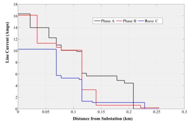
Fig. 4. Feeder Amp profile at the farthest node.
