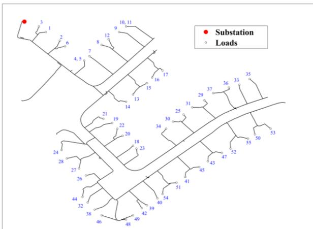
Fig. 1. Test feeder one-line diagram.
