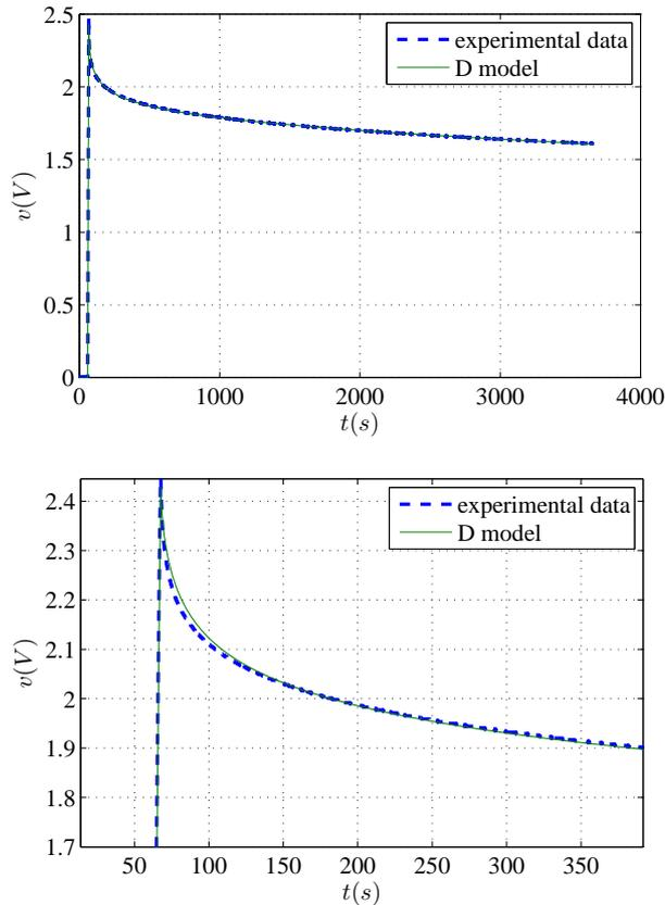
Figure 5: Experimental data and D model for a charge current of  $i = 0.25A$  ( $1F$  EDLC). Whole test at top, and zoomed detail at bottom.
