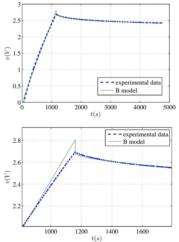
Figure 6: Experimental data and B model for a charge current of  $i = 0.25A$  ( $100F$  EDLC). Whole test at top, and zoomed detail at bottom.
