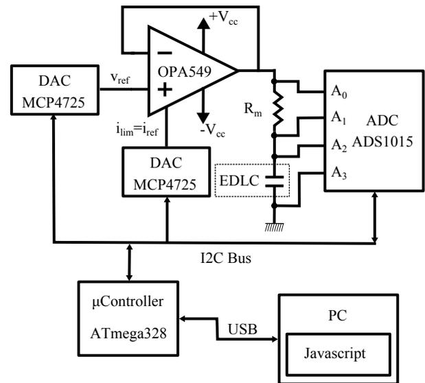
Figure 2: Basic diagram of the identification system.
