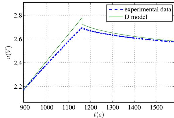
Figure 7: Experimental data and D model for a charge current of  $i = 0.25A$  (100F EDLC). Whole test at top, and zoomed detail at bottom.
