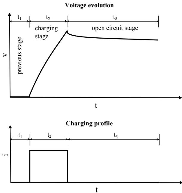
Figure 3: Galvanostatic charge method. Current profile  $i(t)$  at bottom, voltage evolution  $v(t)$  at top.
