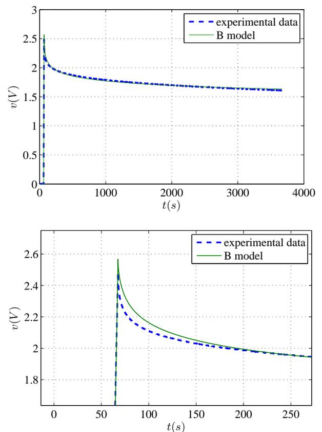
Figure 4: Experimental data and B model for a charge current of  $i = 0.25A$  (1F EDLC). Whole test at top, and zoomed detail at bottom.
