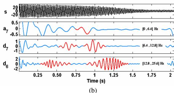
Fig. 4. (a) High-level wavelet signals resulting from the DWT for a healthy machine. (b) High-level wavelet signals resulting from DWT for a machine with 2 broken rotor bars
