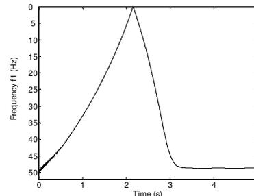
Fig. 3. Variation of the frequency of the left sideband during the startup process for a machine with a broken rotor bar.
