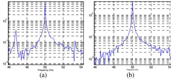
Fig. 1. Classical detection of broken rotor bars. (a) loaded machine (b) unloaded machine
