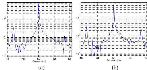
Fig. 2. (a) Sideband components due to broken rotor bars. (b) frequencies caused by fluctuating torque in a healthy machine
