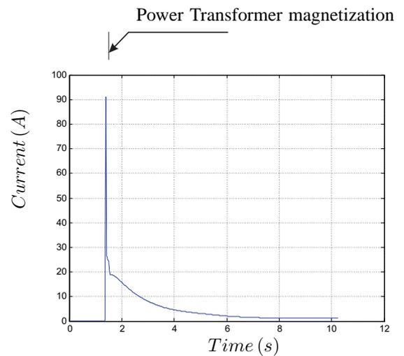
Figure 6. Homopolar current demanded by the power transformer number 2 during the magnetization (rms value).
