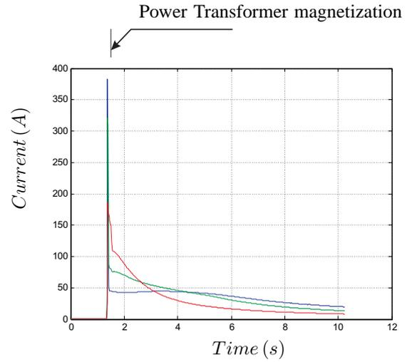
Figure 4. Current demanded by the power transformer number 2 during the magnetization (rms value).
