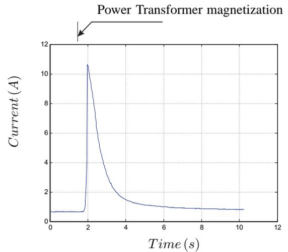
**Figure 9.** Homopolar current supplied by the cogeneration during the magnetization (rms value).
