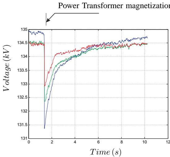
Figure 3. Voltage evolution at 220 kV bus during power transformer magnetization.
