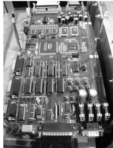
Fig. 6. Photography of the control board based on the TMS320LF2407 DSP
