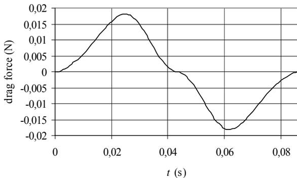
Fig. 5: Time evolution of the drag force in the first period of oscillation for  $\beta = 30^\circ$  and  $\varphi = 0^\circ$  (sphere)
