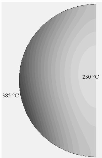
Fig. 10: Distribution of temperature in the sphere for  $\beta = 60^\circ$  and  $\varphi = 0^\circ$ ,  $t = 9$  s,  $T_{\text{ave}} = 300^\circ\text{C}$
