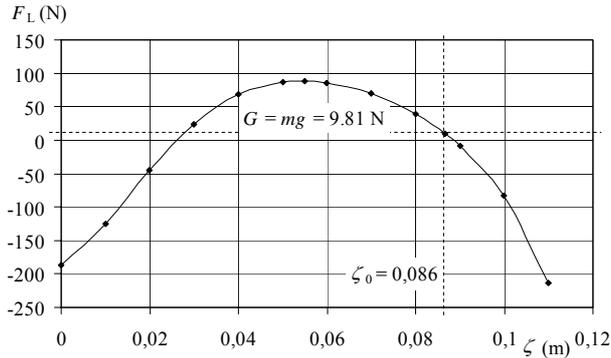
Fig. 8: Static characteristic of the system for  $\beta = 60^\circ$  and  $\varphi = 0^\circ$  (sphere)
