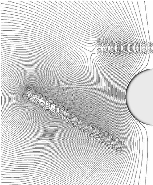
Fig. 9: Magnetic field in the system for  $\beta = 60^\circ$  and  $\varphi = 0^\circ$  (sphere)
