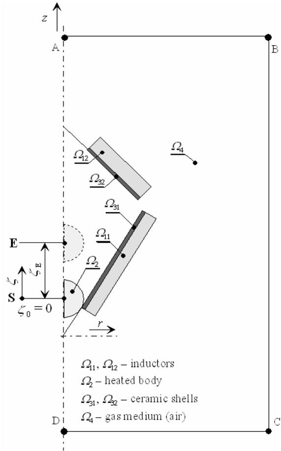
Fig. 2: Definition area of electromagnetic field
