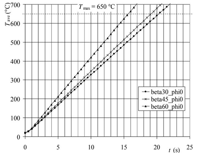
Fig. 11: Time evolution of the average temperature of the cylinder for various angles  $\beta$  and  $\varphi = 0$
