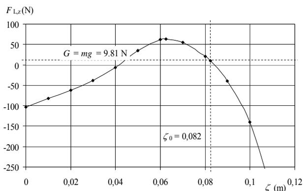
Fig. 12: Static characteristic of the system for  $\beta = 60^\circ$  and  $\varphi = 0^\circ$  (cylinder)
