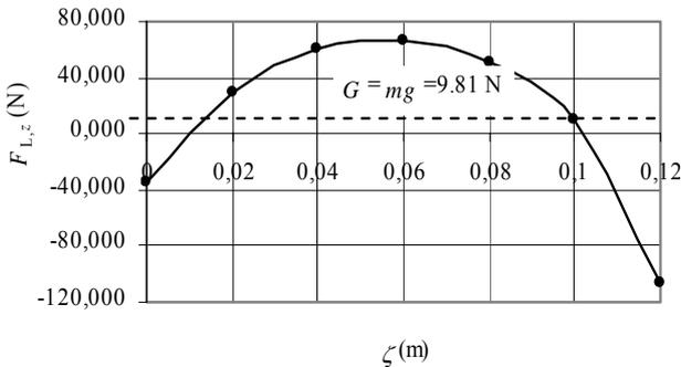
Fig. 4: Static characteristic of the system for  $\beta = 30^\circ$  and  $\varphi = 0^\circ$  (sphere)
