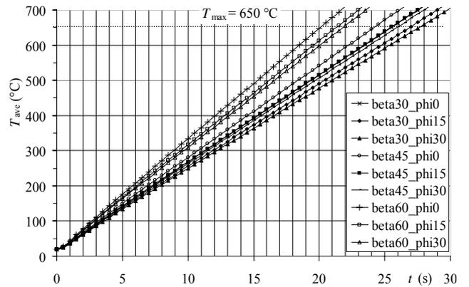
Fig. 7: Time evolution of the average temperature of the sphere for various angles  $\beta$  and  $\varphi$
