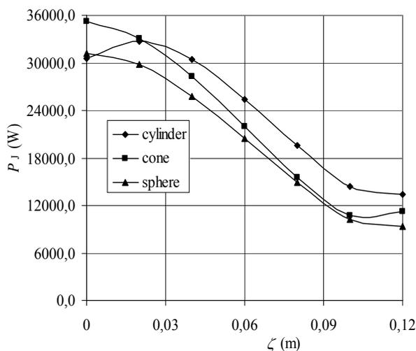
Fig. 13: Dependence of the total Joule losses  $P_J$  produced in the body on  $\zeta$  (for  $\beta = 30^\circ$  and  $\varphi = 0$ )
