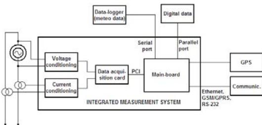
Figure 2: Hardware lay-out.
