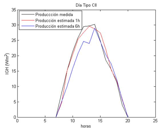
Fig. 2. Comparison of PV power generation measure and forecast for time horizons 1 and 6 hours ahead in C0-Pozo Izquierdo
