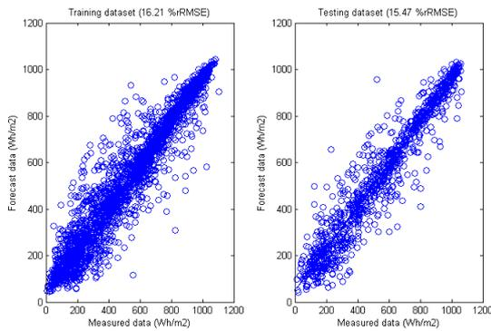
Fig. 1. Comparison of forecasted results with Bayesian Networks and real radiation ground data for C0-Pozo Izquierdo
