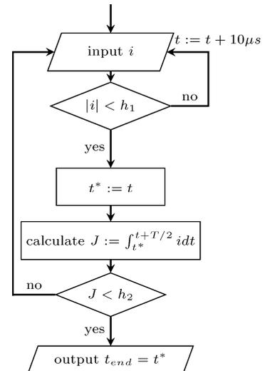
Fig. 6. Algorithm, current termination detection
