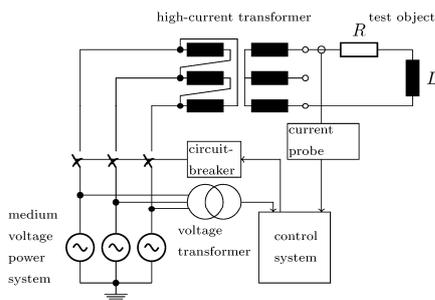
Fig. 1. High-current test setup
