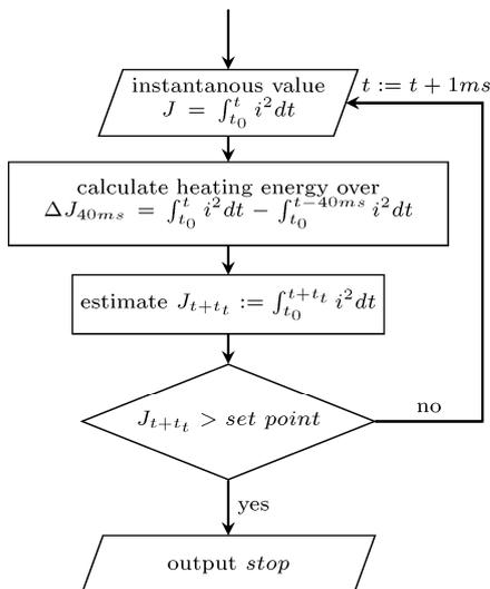
Fig. 4. Algorithm, joule integral prediction
