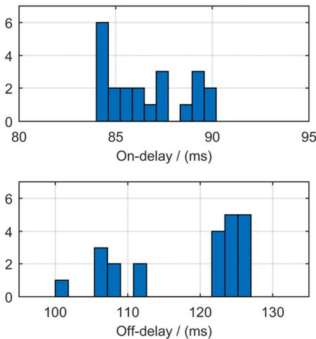
Fig. 3. Distribution of the on- and off-delays of the 3-phase circuit breaker
