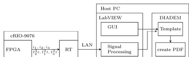
Fig. 9. Signal flow chart of the system
