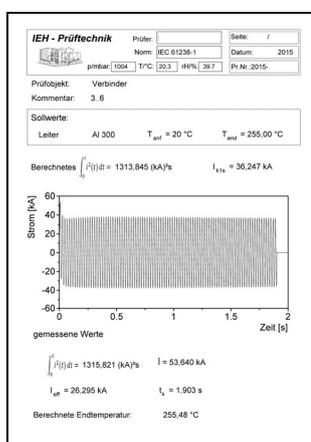
Fig. 14. Example of an automatically generated report, test object: 300 mm<sup>2</sup> aluminium connector
