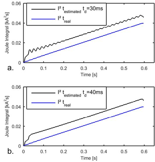
Fig. 5. Joule integral prediction with different slew rate calculations
