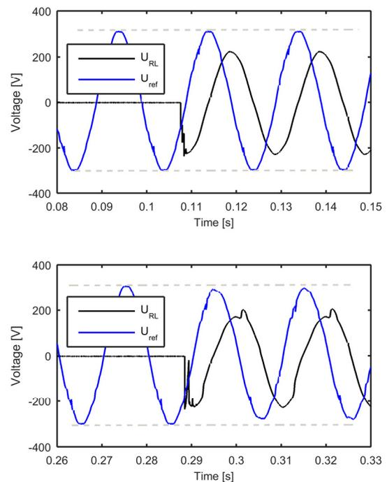
Fig. 12. Experimental test of influence of transformer remanence
