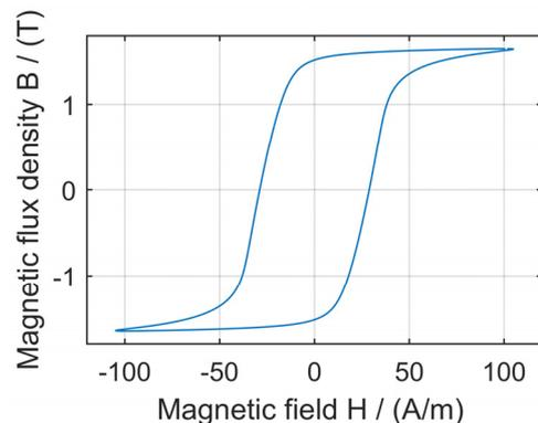
Fig. 2. Magnetic hysteresis diagram of a typical transformer magnetic core
