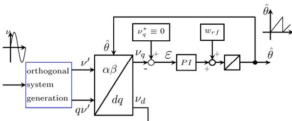
Fig. 7. Single-phase system phase locked loop (PLL) [12]
