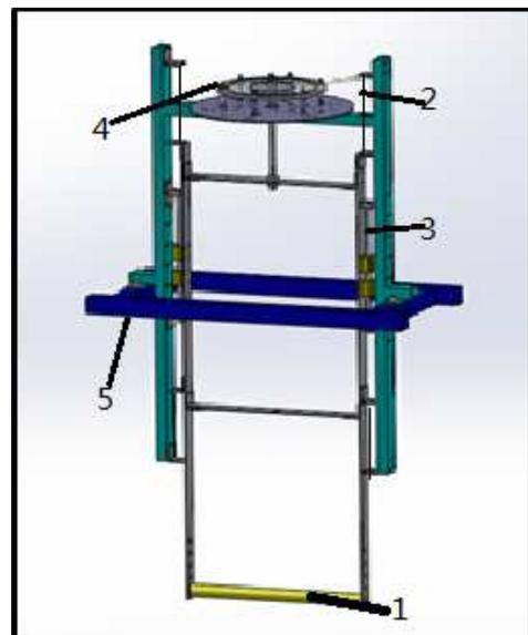
Figure.5 Diagram of the experiment rig: 1-oscillator, 2-spring, 3-rail, 4- transducer unit, 5-fixed frame
