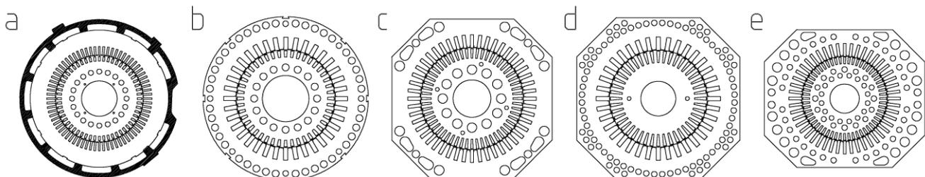
Fig. 1. Laminations for several open (a-c) and encapsulated (d, e) cooling concepts
