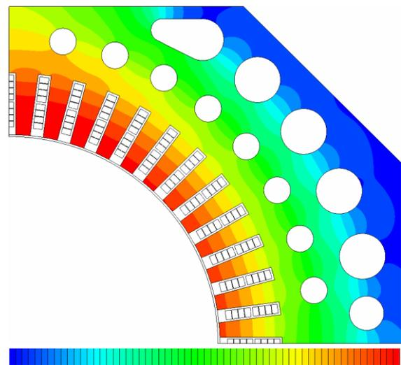
Fig. 8. Finite elements simulation results, temperature dependent thermal conductivity of the electrical sheet, values from 29,8 (blue) to 32,8 W/(m·K) (red)
