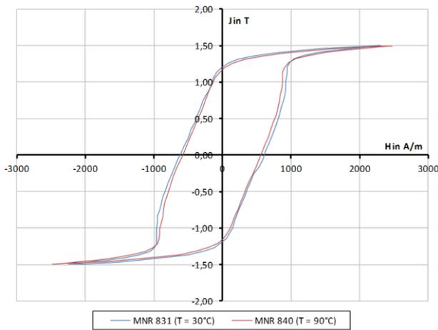
Fig. 6. Hysteresis loop at 30 and 90 °C with a supplied frequency of 1000 Hz [6]
