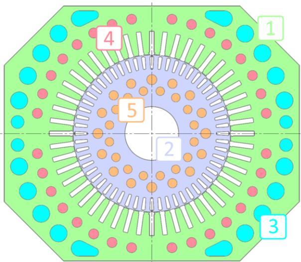
Fig. 3. Sectional view of a lamination of a closed, self-ventilated traction induction machine (DACS cooling concept): 1) stator lamination, 2) rotor lamination, 3) outer stator cooling ducts, 4) inner stator cooling ducts and 5) rotor cooling ducts
