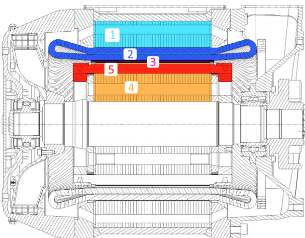
Fig. 5. Longitudinal cross section of an open, self-ventilated traction induction machine: 1) laminated stator core, 2) stator winding, 3) air gap, 4) laminated rotor core and 5) squirrel cage
