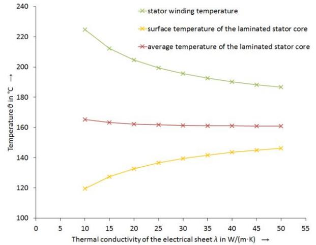
Fig. 7. Thermal conductivity sensitivity analysis of the electrical sheet with a thermal finite element simulation for a traction motor nominal point
