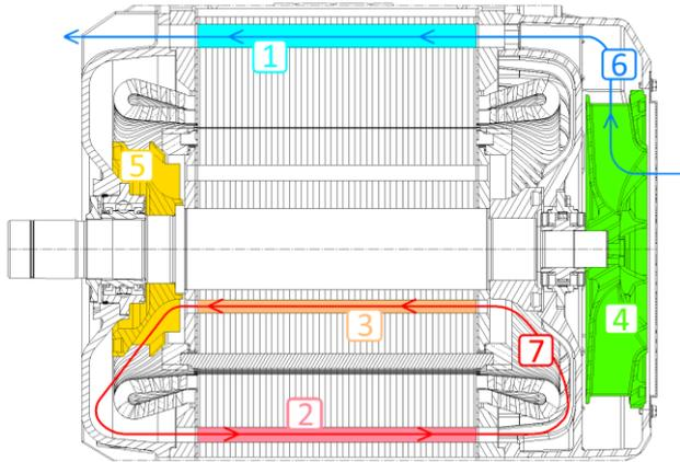
Fig. 2. Longitudinal cross section of a closed, self-ventilated traction induction machine (DACS cooling concept): 1) outer stator cooling duct, 2) inner stator cooling duct, 3) rotor cooling duct, 4) outer fan, 5) inner fan, 6) outer cooling circuit and 7) inner cooling circuit
