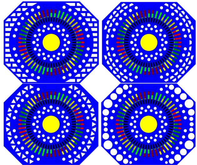
Fig. 4. Sectional views of various lamination designs
