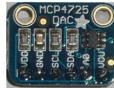
Figure 4: Digital-analogical converter **MCP4725**.
