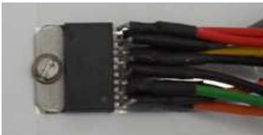
Figure 2: Power operational amplifier **OPA549**.
