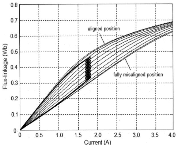
Fig. 3. Magnetisation characteristics.
