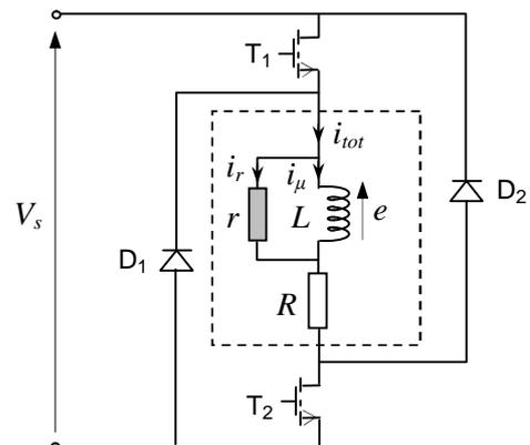
Fig. 2. Functional per-phase equivalent circuit of SR machine.
