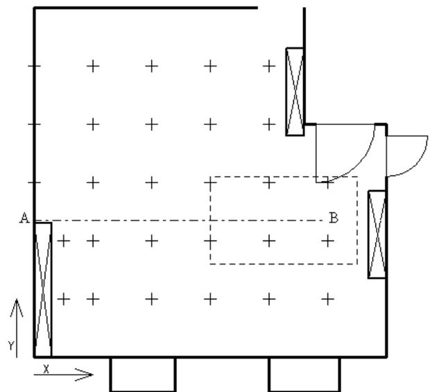
Fig. 7. Top view of the computer room with the spots of the measurements and the iron plate localization
