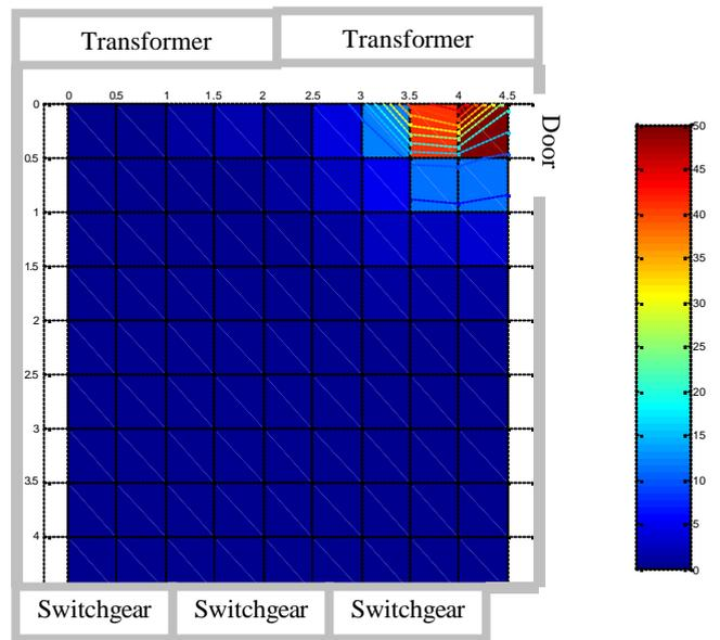
Fig. 11. Room transformer layout with the magnetic field (in  $\mu\text{T}$ ) distribution at 1.1 m, at about 3:30 pm
