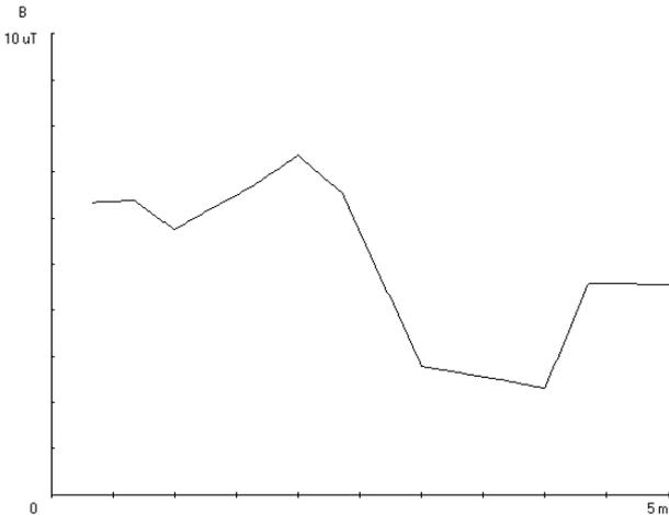
Fig. 14. Variation of the magnetic induction along the center line A-B above the transformer in the computer room floor
