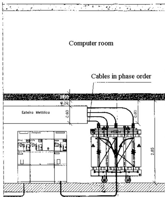
Fig. 6. Front view of the transformer and computer rooms
