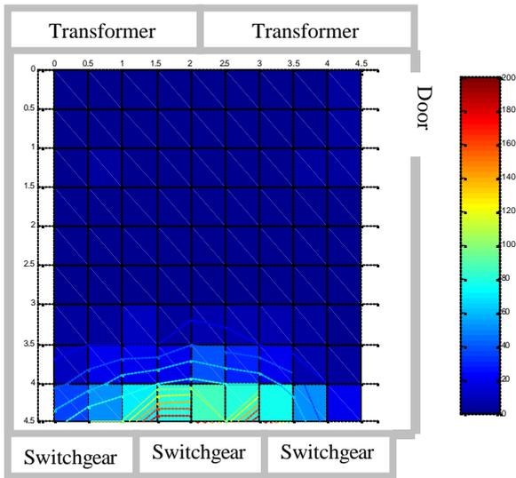
Fig. 9. Room transformer layout with the electric field (in V/m) distribution at 1.7 m, at about 2 pm
