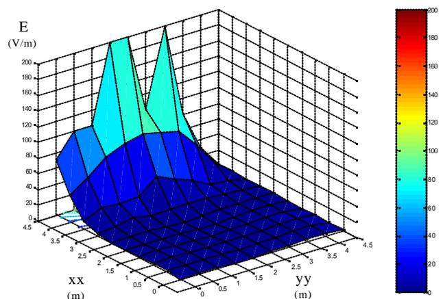
Fig. 8. Electric field distribution at 1.7 m, at about 2 pm
