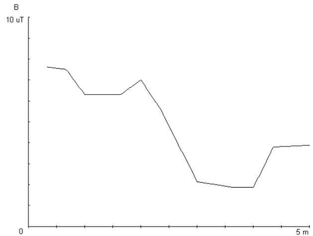
Fig. 15. Variation of the magnetic induction along the center line A-B, 1 m above the computer room floor
