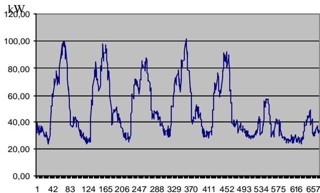
Fig. 3. Weekly load diagram of the transformer plotted with 15 minutes intervals
