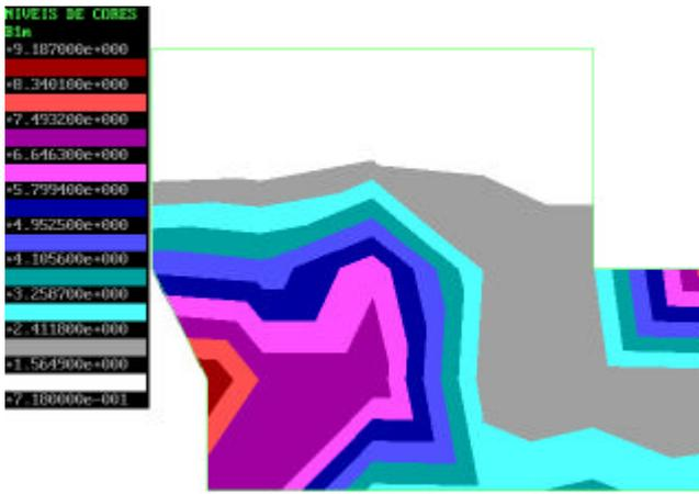
Fig. 13. Amplitudes of the induction B 1 m above the room floor
