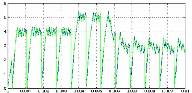
Fig. 11: Estimated and real SRM phase currents
