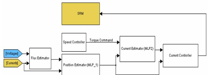
Fig. 12: Block diagram of the SRM drive system
