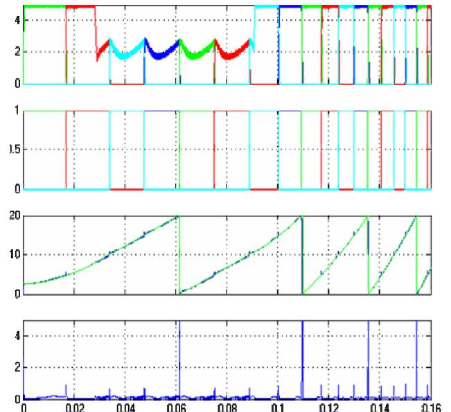
Fig. 8: Simulation for a close loop system working with a neural network for all phases. From top to down: a) Phase Currents with different current command values; b) Excitation pulses sequence obtained from the estimated position; c) Estimated and real rotor position for a complete mechanical cycle between two poles; d) Absolute error between the estimated and real rotor position
