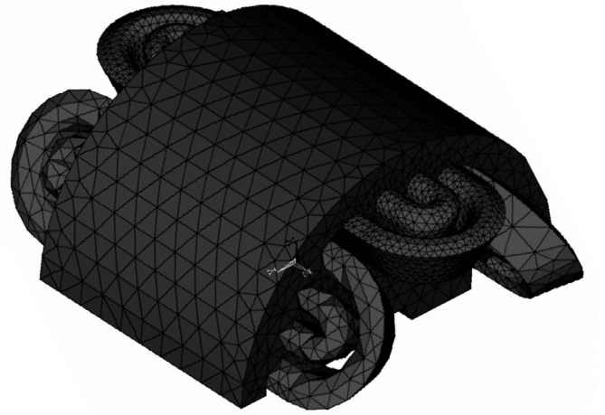
Fig.4. Finite element discretization of the switched reluctance machine.
