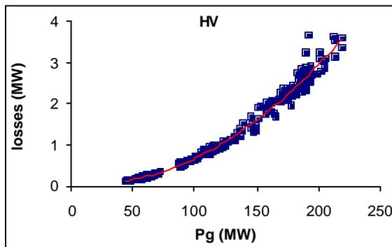
Fig. 6. HV losses as a function of generated power
