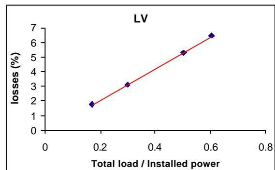
Fig. 4. LV losses (%) as a function of the relation total load divided by installed power
