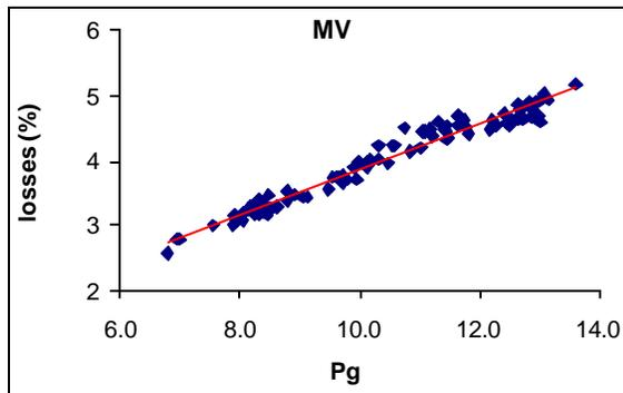
Fig. 5. MV losses (%) as a function of generated power
