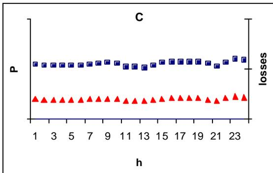
Fig. 9. Diagrams of load (squares) and losses (triangles) for set C (May, workday)
