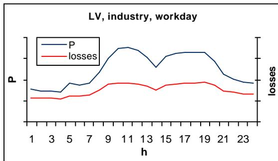
Fig. 11. Load diagram and associated losses for and individual consumer (LV, industrial, workday)
