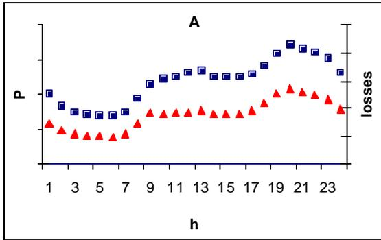
Fig. 7. Diagrams of load (squares) and losses (triangles) for set A (January, workday)
