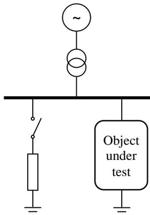
Fig. 2. Sag generator with parallel impedance configuration
