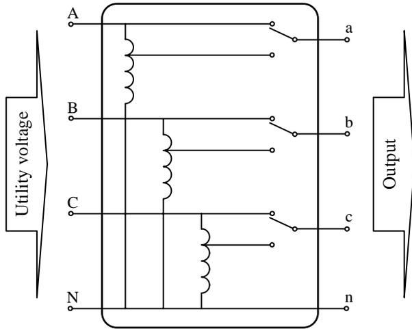
Fig. 1. EPRI's voltage sag generator
