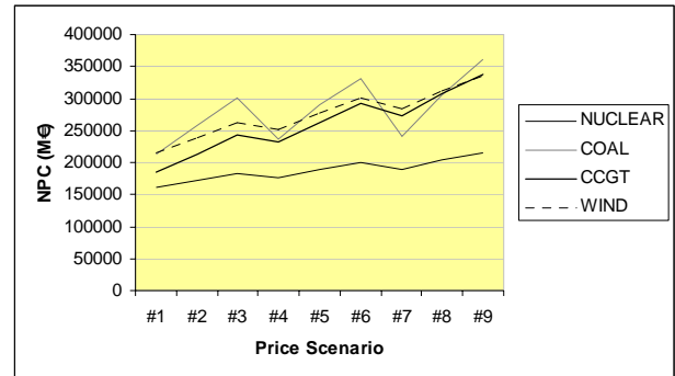
Fig. 3. NPC of each plan in the considered gas and CO 2 price scenarios
