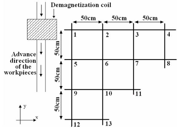
Figure 3 - Map of measurements around the coil.
