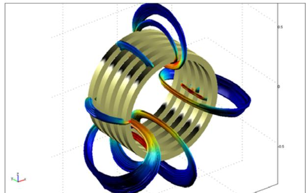
Figure 1 - Coil with workpiece and magnetic flux lines.
