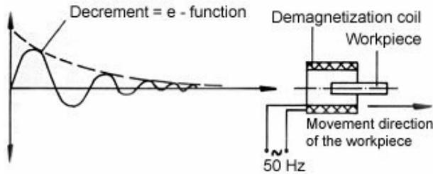
Figure 2 - Demagnetization process.
