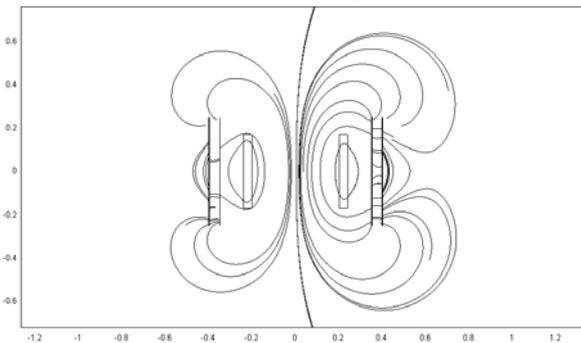
Figure 6 - Flux lines distributions with a second screen.
