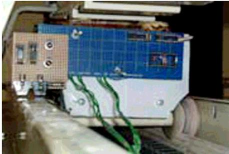
Fig. 6. Optical sensors and frequency-voltage converter
