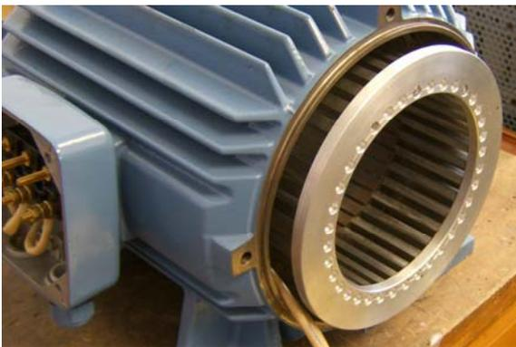
Fig. 1 – Stator of the inverted induction motor.
