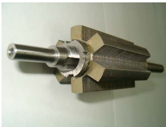
Fig. 3. Rotor of the 8/6 SRM
