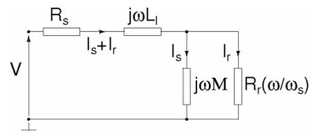
Fig. 1. Simple steady state per phase circuit model.
