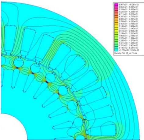
Fig. 2a. Type 2 rotor geometry analyzed by FEMM.
