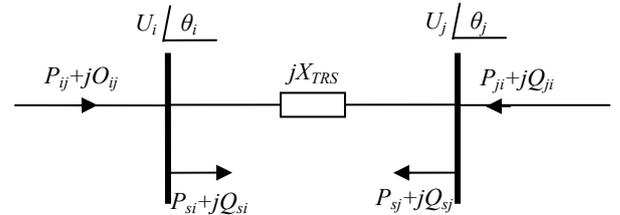
Fig.2. UPFC injection model
