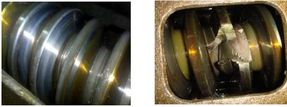
Fig. 2: Detail of a worm showing surface wear (left); detail of a broken worm (right).
