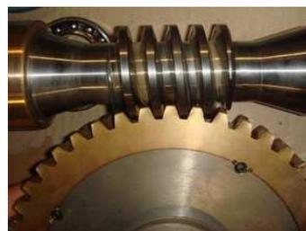
Fig. 1: Worm gears.
