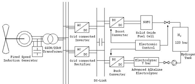
Fig. 1. Schematic of the modelled wind farm with hydrogen storage system.
