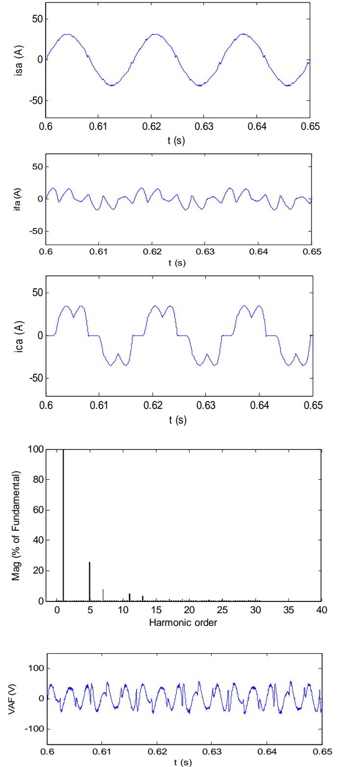
Fig. 3. Simulation results for the proposed control scheme (phase a). From top to bottom: Source current  $i_{sa}$  (A), Filter current  $i_{fa}$  (A), Load current  $i_{la}$  (A), and Active filter voltage  $V_{AF}$  (V).
