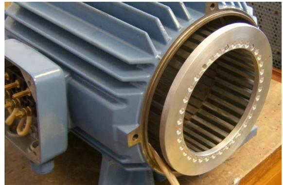
Fig. 3– Stator of the inverted induction motor.
