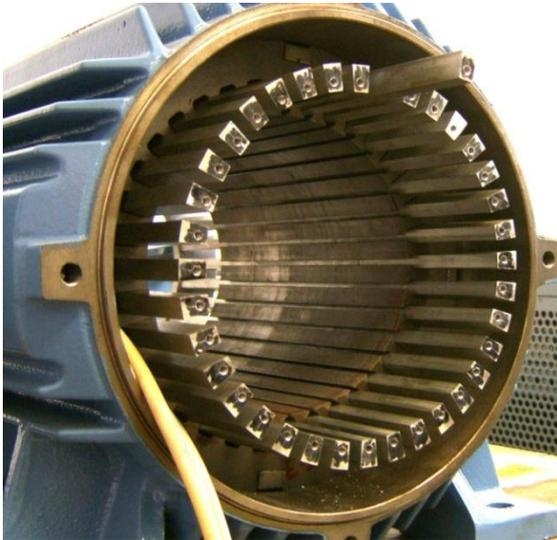
Fig. 1 – Bars placed in the stator slots.
