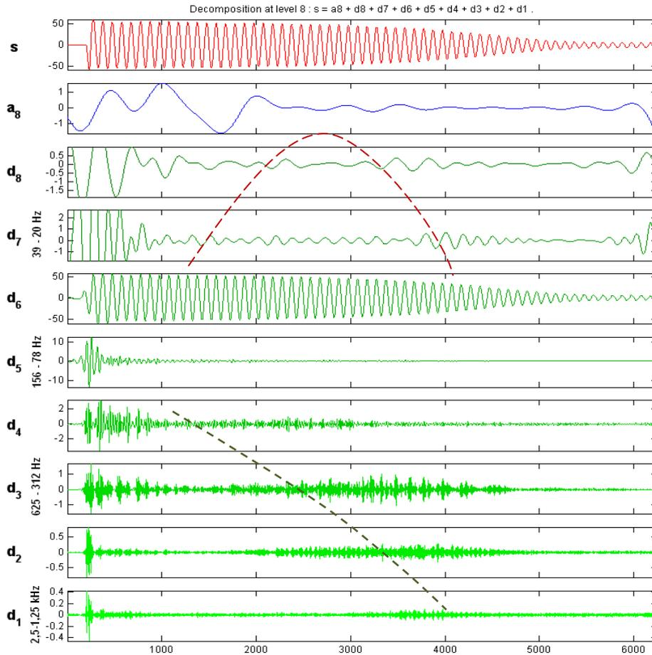
Fig. 8 –Wavelet decomposition of the current startup transient
