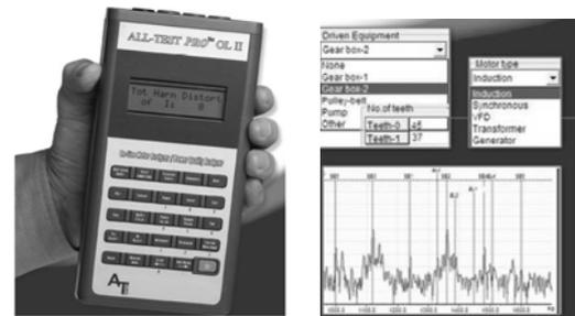
Figure 2. Industrial Equipment to detect failures in motors.
