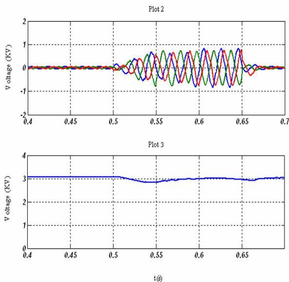
Fig.10. Response of DVR port during fault
