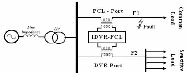
Fig. 6. Schematic diagram of the study system
