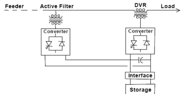
Figure 3. Custom Power based on two Voltage Source Converters and Storage
