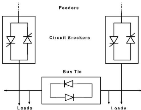
Figure 4 Basic structure of STS.
