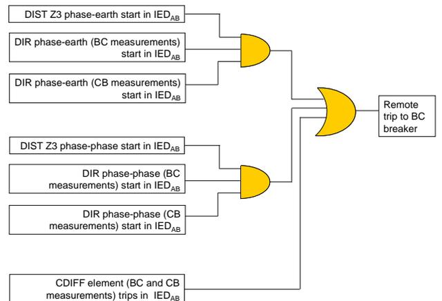
Figure 6. Remote trip logic based in differential, distance and directional elements
