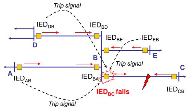
Figure 2. Scheme behaviour against fault and IED failure
