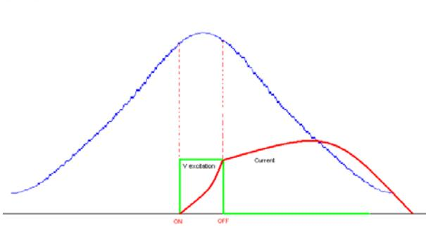
Figure (3) proposed firing angle
