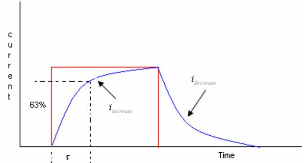
Figure (1) current behaviour inside a winding coil
