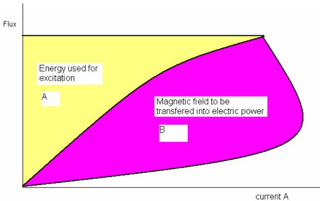
Figure (8) energy conversion in the SR Machine
