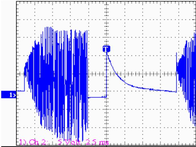
Figure (15) excitation under higher voltage source using a chopping circuit
