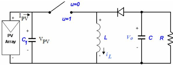
Fig. 5. Buck-boost converter
