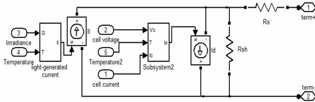
Fig. 2. Equivalent circuit of a PV cell
