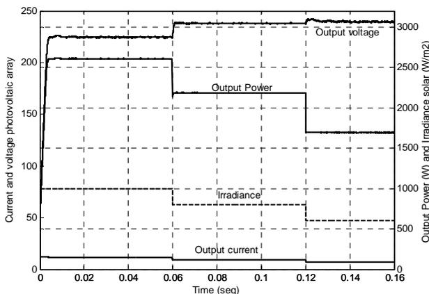
Fig. 10. Evolution of  $V_{PV}$ ,  $I_{PV}$  and  $P_{PV}$
