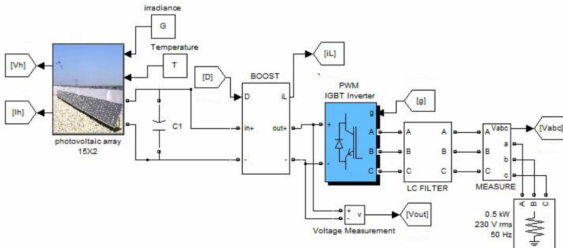
Fig. 7. Photovoltaic array interconnected to AC load
