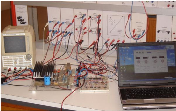
Fig. 2. Dual source prototype during experimental performance tests.
