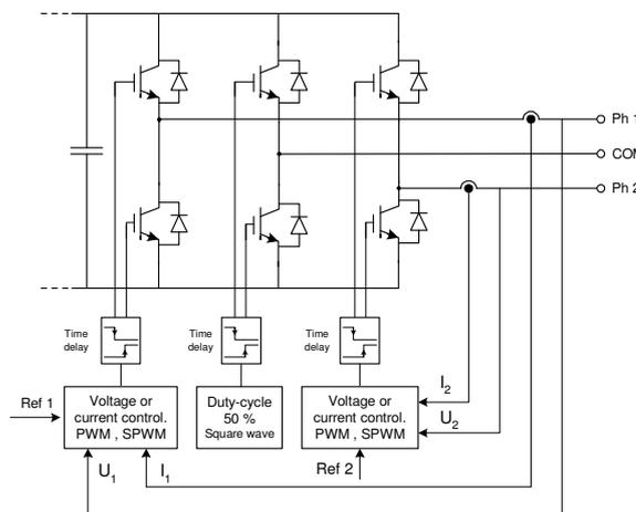
Fig. 1. Power source diagram using three-leg inverter.
