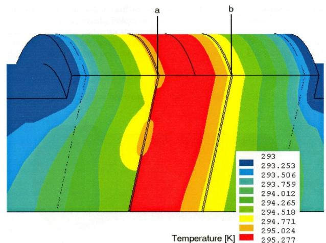
Fig. 4 Temperature distribution within the contact body
