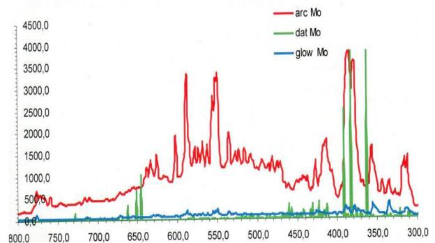
Fig. 6 Contact compound made of molybdenum (Mo): arc – arcing discharge, glow – glowing discharge, dat – data from physico-chemical tables; abscissa – wavelength, ordinate – radiation intensity
