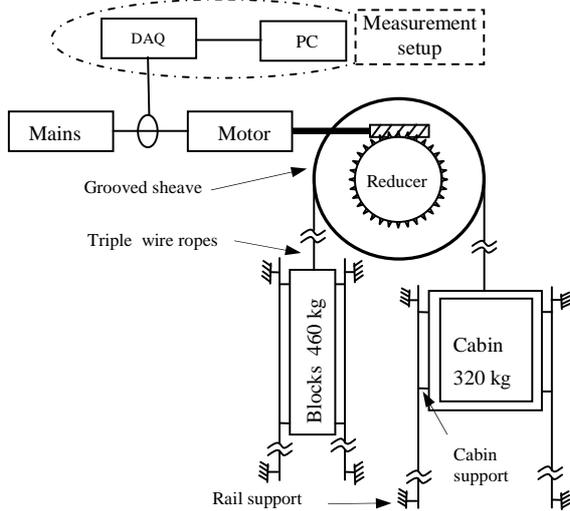
Fig. 1: Classical elevator system and measurement setup.
