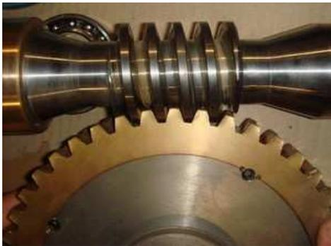
Fig. 2: Worm gears.
