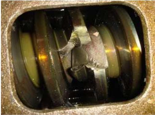
Fig. 4: Detail of a broken worm.
