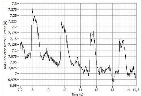
Fig.6: The induction motor current was measured at 1400 RPM.
