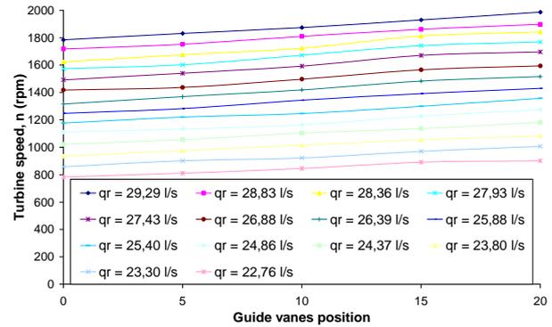
Fig. 12: Closed loop steady-state measurements (turbine speed).
