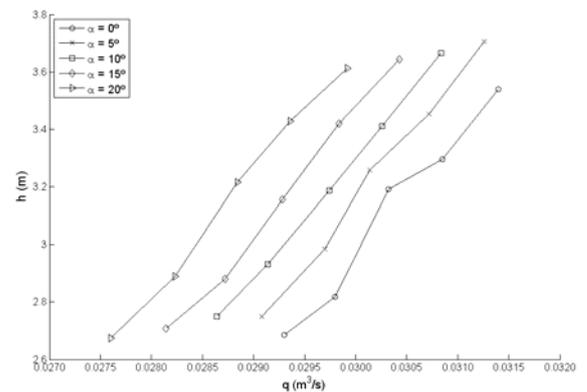
Fig. 3: Head-discharge curves for turbine speed  $n_t = 2000$  rpm.
