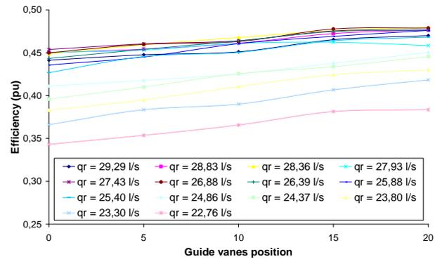
Fig. 13: Closed loop steady-state measurements (turbine efficiency).
