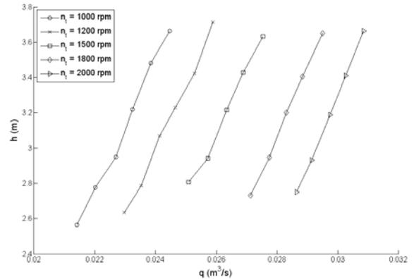
Fig. 2: Head-discharge curves for guide vanes position  $\alpha = 10^\circ$ .
