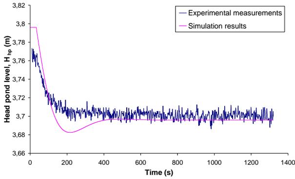
Fig. 11: Head pond level with (PI) control ( $\Delta h_{ref} = -0.033$  pu).
