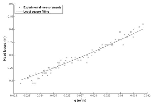
Fig. 6: Head losses in the head-race conduit.
