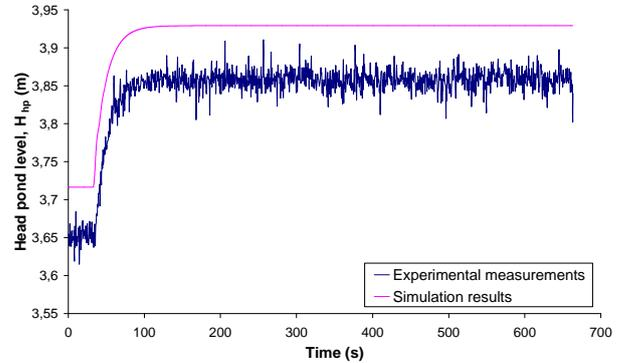
Fig. 9: Head pond level with (P) control ( $\Delta h_{ref} = 0.080$  pu).
