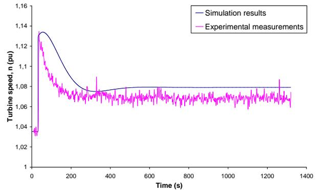
Fig. 10: Turbine speed with (PI) control ( $\Delta h_{ref} = -0.033$  pu).
