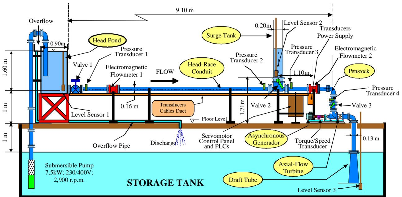
Fig 4: Laboratory plant layout
