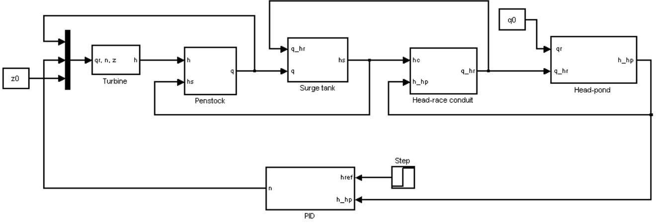
Fig. 7: Block diagram of the primary control loop.
