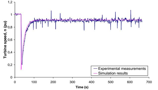
Fig. 8: Turbine speed with (P) control ( $\Delta h_{ref} = 0.080$  pu).
