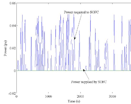
Fig. 7. Power required and supplied by the fuel cell.
