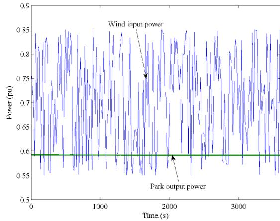
Fig. 6. Response of the wind farm when required setpoint power is lower than actual wind input power.
