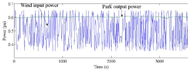
Fig. 4. Response of the wind farm when required setpoint power is greater than actual wind input power.
