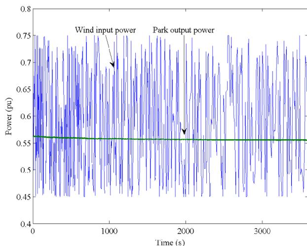
Fig. 8 Response of the wind farm when required setpoint power equals to actual wind input power.
