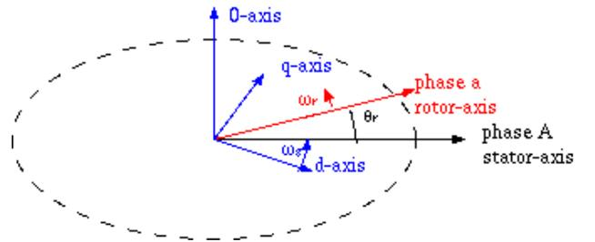
Fig. 2. Induction machine windings in the  $dq0$  arbitrary reference frame.
