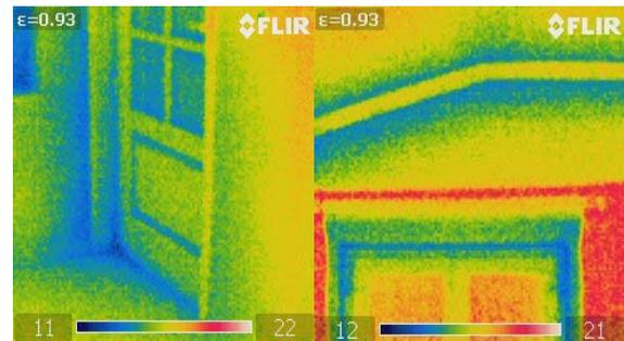
Figure 2 - Door, Ceiling and Window Thermal Leaks.
