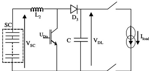
Fig. 2. Discharging SCs to the load
