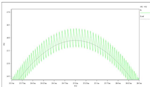
Fig. 11: DC link current wave form
