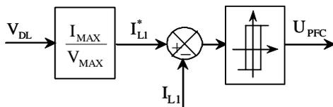
Fig. 6: Control of the boost converter
