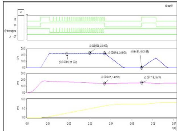
Fig.13: Control of the SC converter, charging authorization, SCs current, condition on the charging SCs voltage, SCs current, DC link voltage and the SCs voltage
