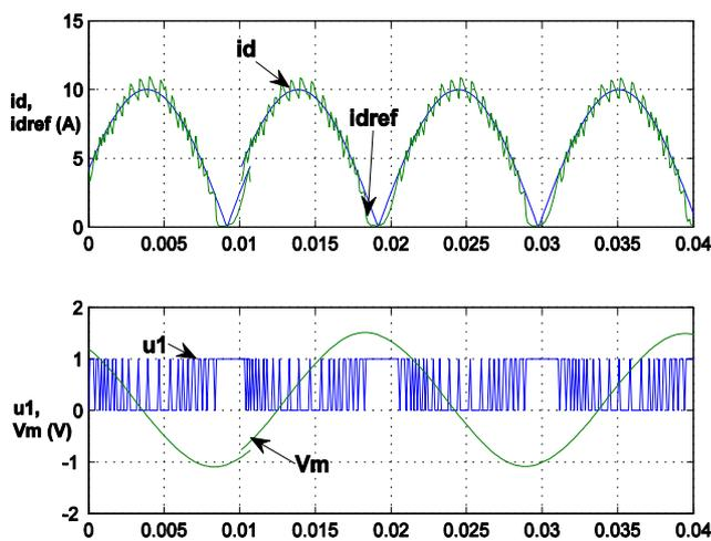
Fig. 16: Experimental Waveforms for currents, control and voltage ( $V_m/10$ ).
