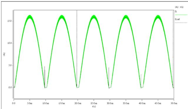
Fig. 10: Inputs boost current – reference and measured values
