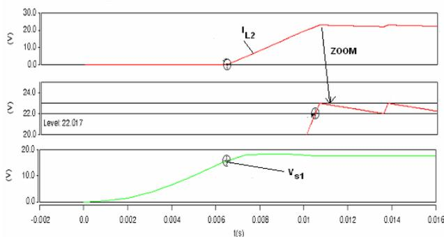
Fig. 12: SCs current and voltage
