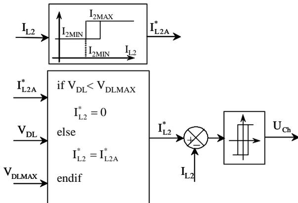
Fig. 7: Control of the SCs converter
