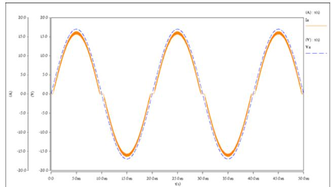
Fig. 9: Rectifier phase current
