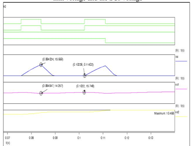
Fig.14: Control of the SC converter, charging authorization, SCs current, condition on the charging SCs voltage, SCs current, DC link voltage and the SCs voltage
