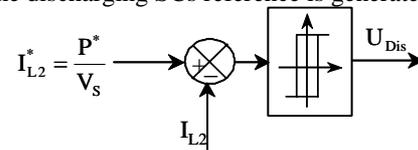
Fig. 8: Control of the SCs discharging
