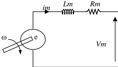
Fig 4. Single phase machine model
