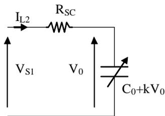
Fig. 5 Supercapacitor electrical model
